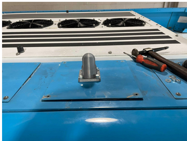
Photo of the Antenna Dome on Top of the Bus
